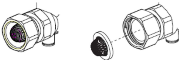
Water Filter In-place
