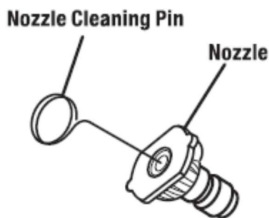
Nozzle cleaning pin – Anneau de nettoyage de la buse nozzle – Buse
